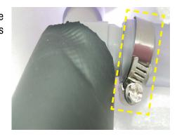
• Also, ensure that the Blower Check Valve, located under the Control Pack, is tightly secured. These can sometimes become dislodged during shipping, and cause tub malfunctions.
